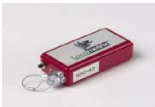
Sensor-recorder for the walk and the run. Maximum duration of recording of 7 hours and 45 minutes, frequency 100Hz, 3 axes, 6 g sensitivity, data transfer via USB.
